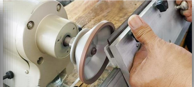
7) Sharpen Electric Planer blade
